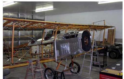
The Jenny in the Doyle hanger, April 2004. The wings are attached, and all flight control surfaces are installed. The flight control rigging is in progress.
